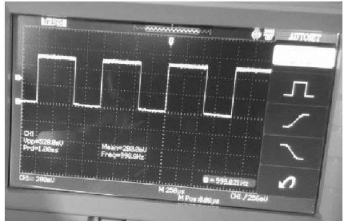
Fig. 10: Switching Waveform of Upper MOSFET
