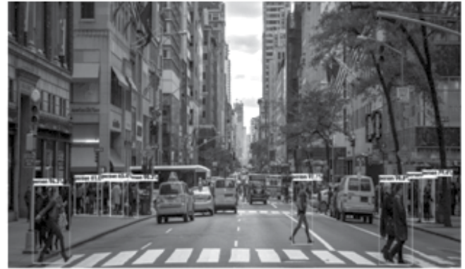
Figure.5: Output of object detection model on human object detection
