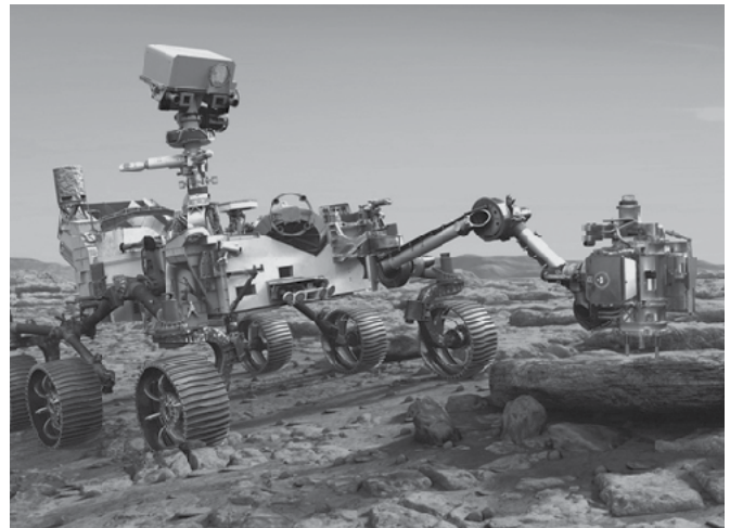
The Perseverance Rover drilling into Dark Rocks for collection of Martian Samples.
