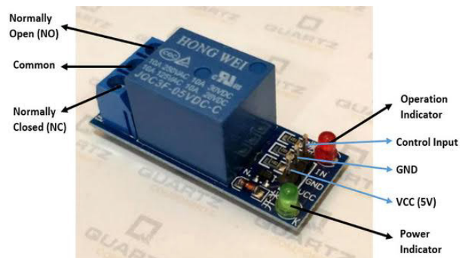
Fig. 8 Power Relay Module
