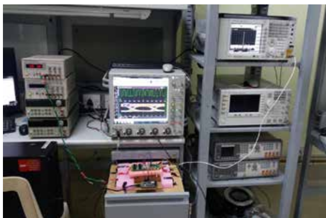
Test and measurement structure to test the On-Chip Jitter
