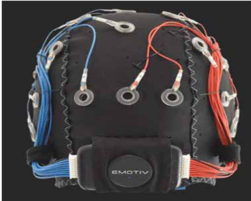
Channel Gel Wireless EEG Head Cap System for collecting high-density EEG signals and 14-Channel Wireless EEG Headset of EMOTIV's industry.
