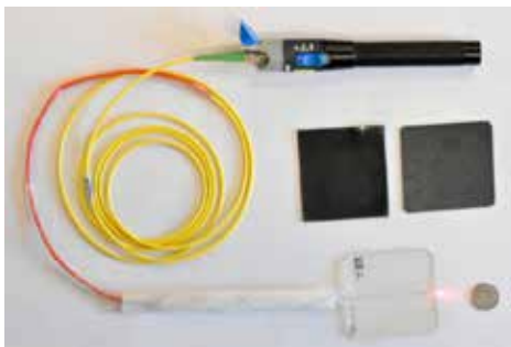
FBG-based physiological sensor element sandwiched between PDMS polymer material
