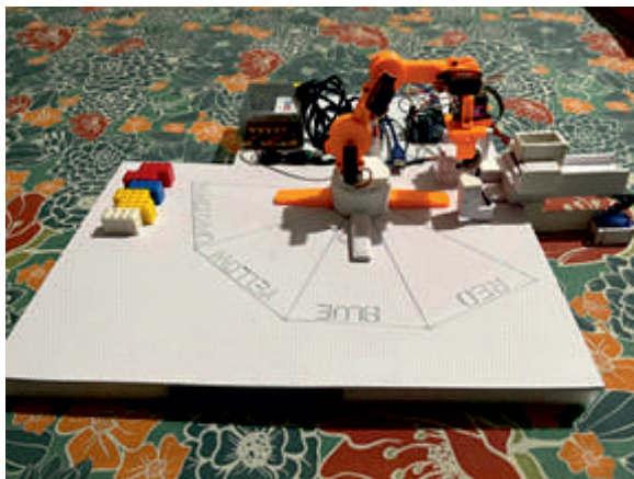
Fig 7 Prototype of the 5 DOF Smart Robotic Arm
